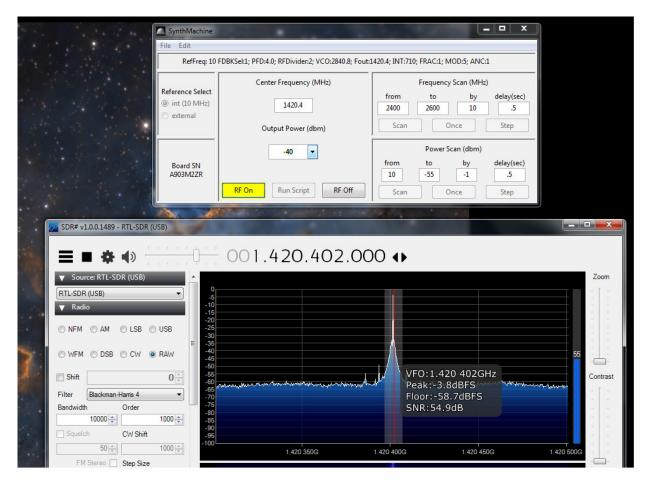
On the top is the window that runs the generator, set to 1420.2MHz with an output level of -40dbm below the SDR# software showing the peak output at -3.8dBFS which indicates that the receiver has a gain of 36.2dB. This of course is for a single frequency. If you need to plot data for a range of frequencies, or a spectrum, measure multiple data points and record in a program such as Microsoft Excel, then graph the data.
