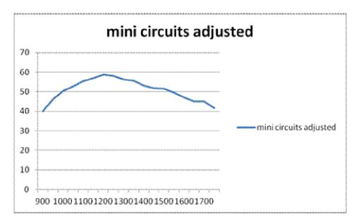
To run the test, first the TPI was connected directly to the RTL-SDR and a reading was taken every .5 Mhz from 900MHz to 1750MHz (the limit of the RTL-SDR) and recoded on a spread sheet. Then the same readings were taken through the amplifier/filter chain. The difference in the readings for each point were then plotted to determine the gain and bandwidth of the chain.
